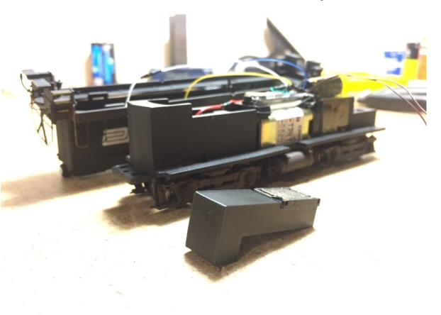
The Loksound Select Micro decoder was installed. Here is the Scale Sound Systems speaker system ready to install. It fits snuggly down into the frame hovering over the front truck tower.
