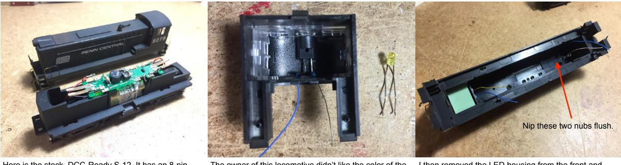
Here is the stock, DCC-Ready S-12. It has an 8-pin decoder receptacle, but no room for a speaker or capacitor if we keep the factory PCB. The bronze tabs sticking off the front of the PCB contact a fitting for the front LED headlight.
