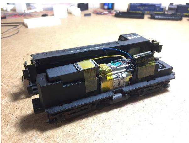
Here's the finished install. Both pairs of headlight wires are equipped with Pin & Socket Micro Connectors so that the shell can be fully freed from the mechanism. A 16V, 2200uF capacitor sit's down into the frame just behind the motor and in front of the cab interior. It is also equipped with a single Pin & Socket Micro Connector so the capacitor can be bypassed for any future Lokprogrammer programming.
