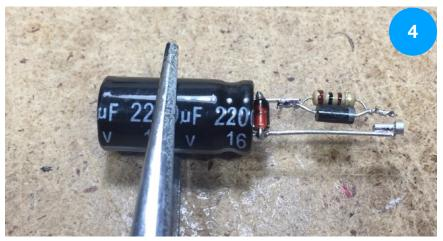
Finally, slip some 1.5mm heat shrink over the negative lead and tighten it down with a clean soldering iron.
