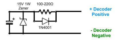
Start the assembly by soldering the Zener diode to the capacitor's leads. Be sure to orient the Zener's cathode (stripe) to the capacitors anode (positive). Trim the Zener's excess leads.
