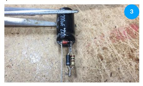
Tin and solder the micro-pin socket to the capacitor's negative lead.
