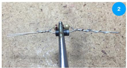
Tin & solder the resistor/diode assembly to the capacitors positive lead.
