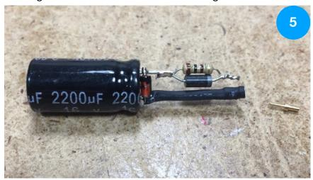
As shown here on the left, after you solder the Zener to the capacitor, you can bend the capacitor's leads back on itself and finish the final assembly for a more compact stay-alive.
