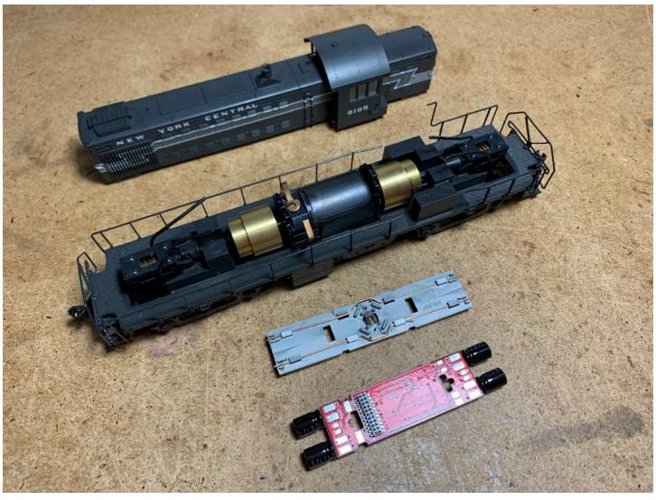
Here we're ready to install the TCS AK-MB1. Strip & tin the four truck-wires and solder short lengths of wire to all four, extending the length an inch or two. Heat-shrink the joints.
