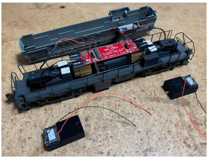
Here we see the four truck-wires extended with their joints sealed in heat-shrink. The motor's copper strips were close enough to the TCS motherboard pads that I simply bent them to comfortably lay over the pads and soldered them directly to the board. Be sure you bend the strips to comfortably line-up; you don't want these stressed. Alternatively, trim the brass strips short and solder wires to them and the motherboard.
