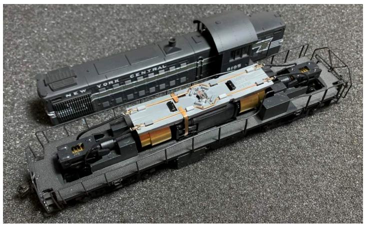
Trim the four truck-wires from the factory "board" and release the two copper motor-strips. Discard the factory "board".
