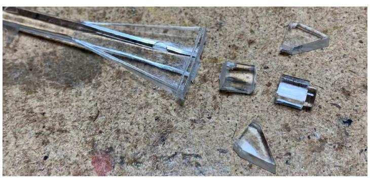
I used a thin Exacto saw to cut the lightpipe into the pieces shown. The only thing I am using here is the headlight lens that fits into the shell. The way I did the lighting, the headlight and number boards all light up together. If you want separate number board lighting, you can install 0402 or 0603 LEDs behind each board in the shell.
