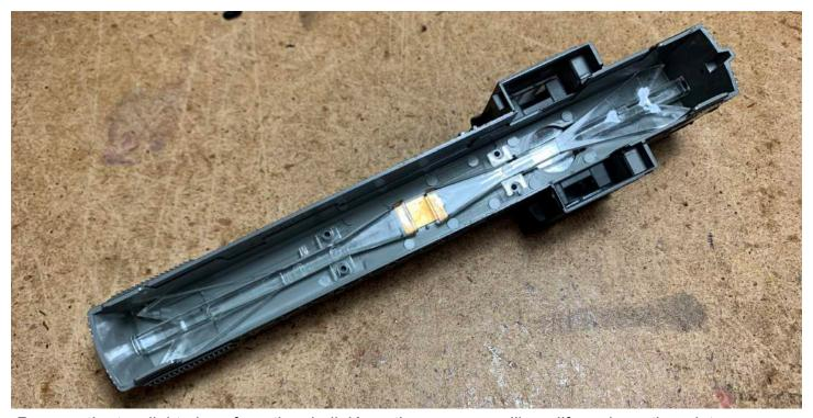
Remove the two light pipes from the shell. Keep these, as we will modify and use them later.
