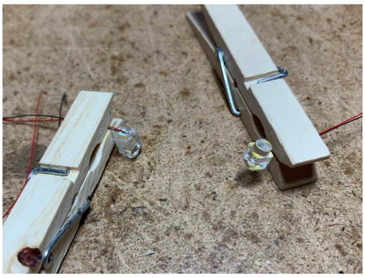
Taking the lenses I trimmed from the stock lightpipes, I glued on 1206 warm-white LEDs.
