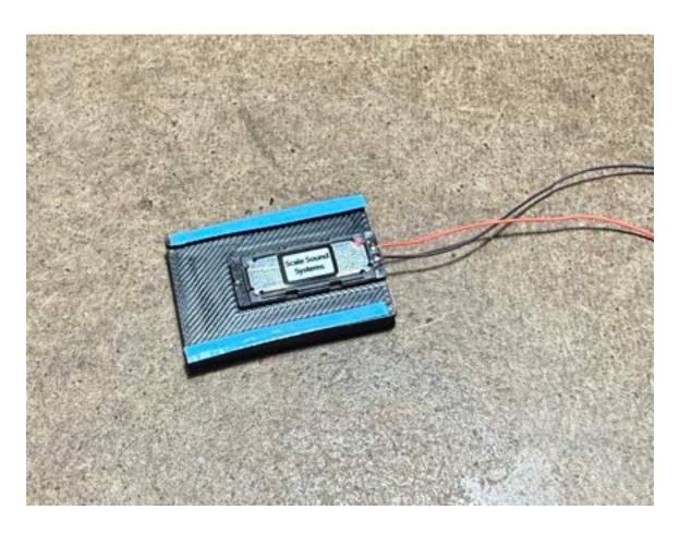
Prepare the SXTH-JBB1 boiler speaker by soldering a couple inches of 36AWG wire to the solderpads. Note that the red-dot indicates the speaker's absolutepositive pad.
