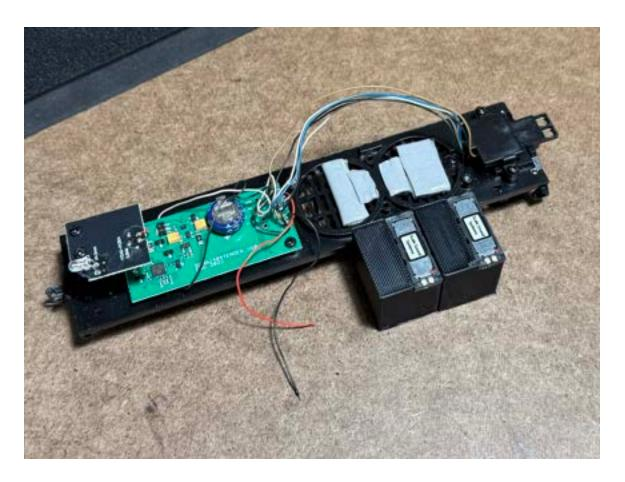
The process is the same if using the  $5.3\Omega$  3-speaker set with twin-FFRC-2025 speakers. You will wire these two speakers in series. This is critical! Wiring them in parallel will result in a  $2.6\Omega$  total load when combined with the boiler-speaker. A 2.6Ω load will destroy any brand of DCC decoder!
