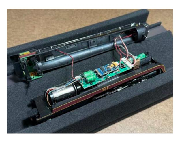
Rest the PCB back into position and install the two screws used to secure it. The SXTH-JBB1 speaker may lift the PCB a little bit but this poses no problem. Plug the decoder back to the board.
