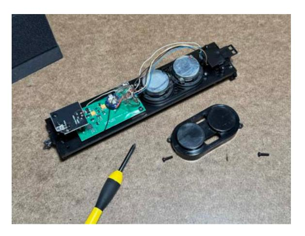
Remove the two screws that secure the speaker enclosure.
