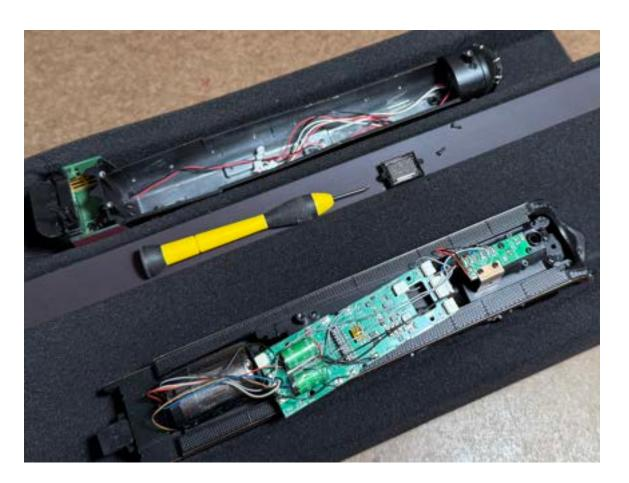
With the motherboard loose, remove the two screws that secure the stock speaker. We will not be reusing the speaker or these screws.
