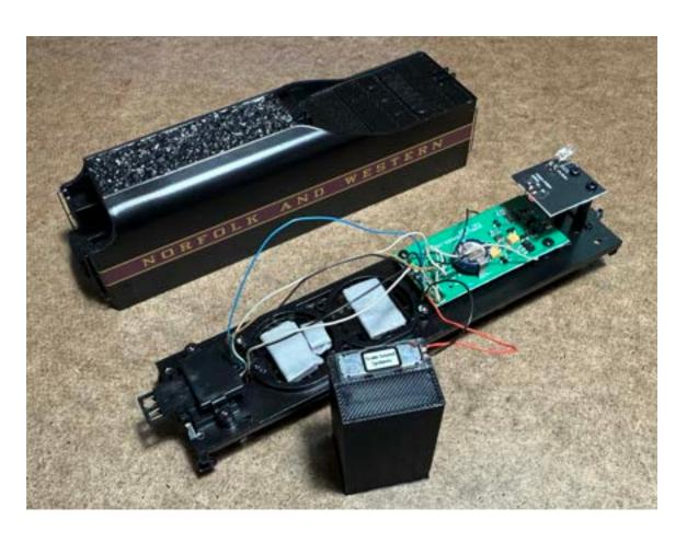
I used thicker, 3M outdoor mounting tape folded and stuck into the frame recesses.
