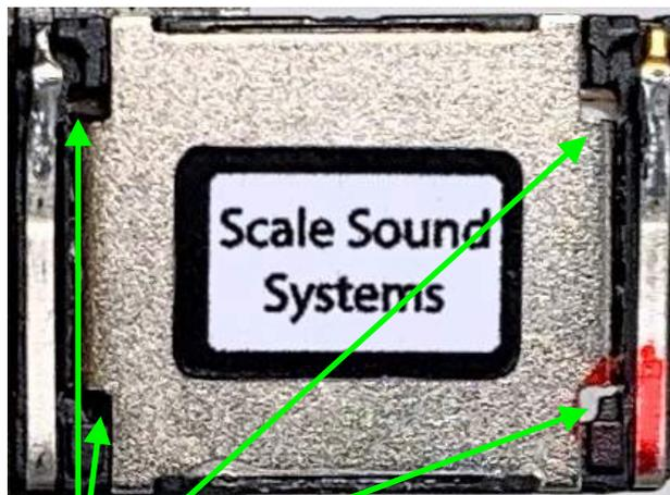
**Use Kapton tape to secure speakers and do not cover the driver's ports.**
