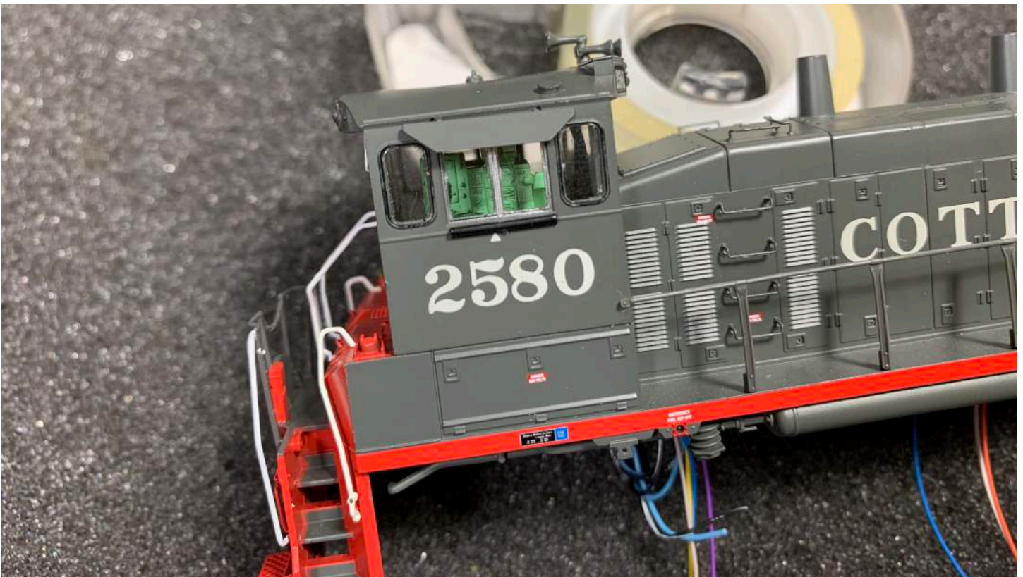
Remember when I promised you would never notice the slight rear-ward control stand positioning? I am a man of my word. The cab interior looks just as “roomy” as before with no wires or KeepAlive® to be seen!
